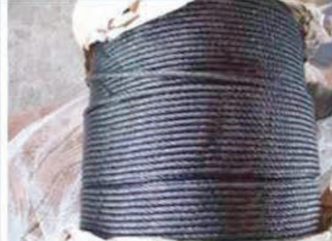
The surface of ungalvanized wire rope
